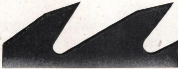
A. FOR HIGH-SPEED RIPPING.
